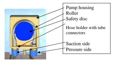
Note Do not twist the hose during assembly For the change of the dosing tube remove the cable strap carfully from the tube nozzle and push on the ends of the new hose to the nozzles. Pay attention that the marks at the ends of the hose are in front of the hose kit and not twisted! Fix again the hose ends by means of the new cable straps. Fit the hose kit as discribed above.
